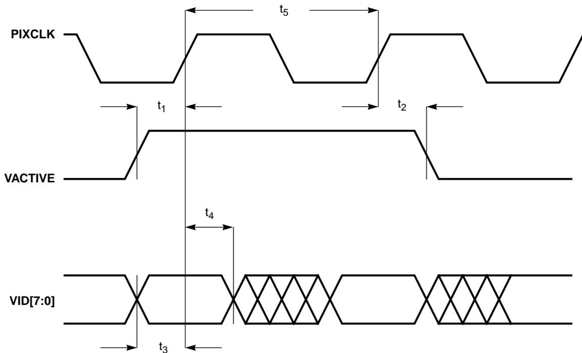
**Figure 6-6. YUV Port (VMI Video) Timing**
