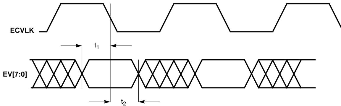
**Figure 6-7. TV Encoder Out Timing**
