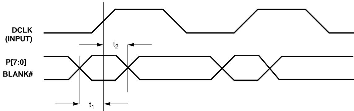
**Figure 6-4. Feature Connector Input**
