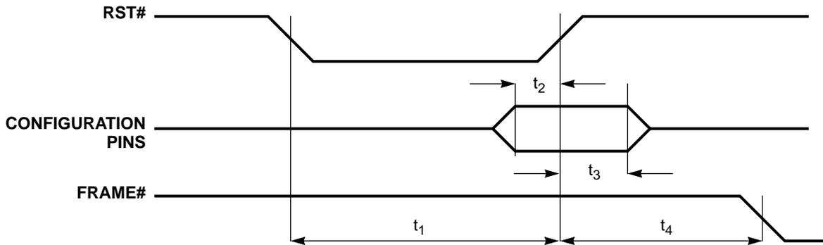
**Figure 6-9. RESET Timing**
