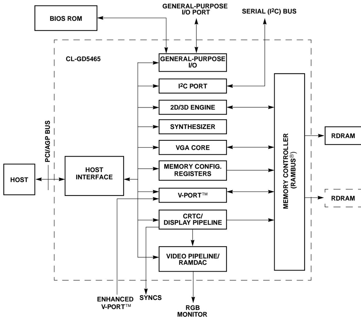
Figure 3-1. CL-GD5465 Block Diagram
