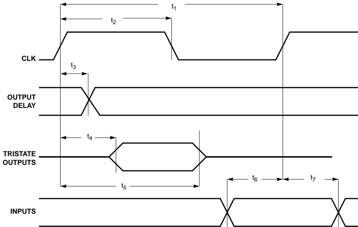
**Figure 6-1. PCI Bus Timing**
